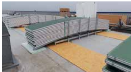
Production of the cassettes in the factory in Zevenbergschen Hoek NL. The lower polycarbonate sheet - with the plastic profiles ( spacers) - is placed on the padded bench.
