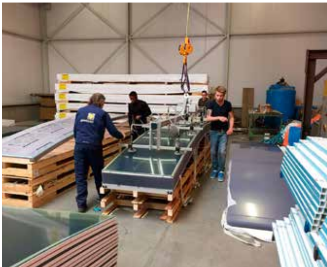
Production of the cassettes in the factory in Zevenbergschen Hoek NL. The lower polycarbonate sheet - with the plastic profiles ( spacers) - is placed on the padded bench.
